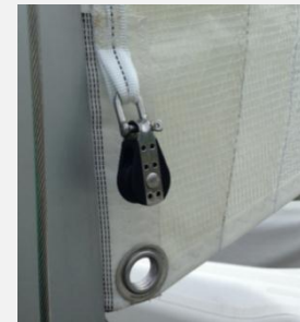
Detail: Loops at the mainsail to fix the new TOPCAT Cunningham ambition
